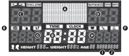
Pressing the Enter/Mode button during use will change heart rate to distance and calories to steps.
