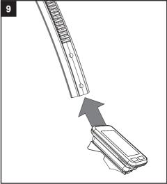
**Computer Assembly:** Slide computer console bracket onto frame bracket from bracket base.
