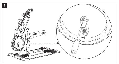
**Transmitter Assembly**: Secure transmitter cover using supplied screws.
