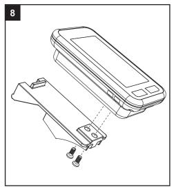
**Computer Assembly**: Attach console bracket to computer console.
