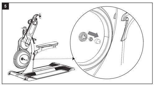
Transmitter Assembly: Remove nut cover and nut on flywheel.
