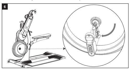
**Transmitter Assembly**: Remove transmitter cover and secure transmitter plate onto flywheel and replace nut. Rotate transmitter down as shown. Do not overtighten. Tighten just until thread passes the Nyloc.
