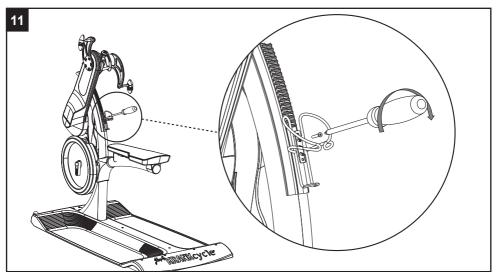
**Frame Bracket Assembly**: Place Bracket onto frame and water bottle cage onto bracket; replace water bottle cage screws with the screws provided. Secure new warning decal over existing decal so that it's clearly visible.
