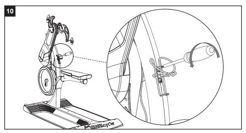
Frame Bracket Assembly: Remove screws from water bottle cage and remove cage.
