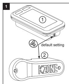
The channel transmitting the cadence signal from the transmitter to the computer console is preset. A sticker on the housing indicates the preset channel on the computer & transmitter.
