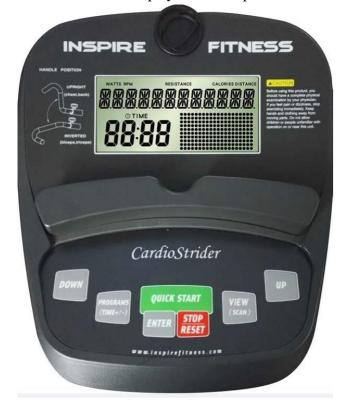
• VIEWING WORKOUT DATA: During a workout RPM and CALORIES are displayed on the scrolling text bar. Press the "VIEW" button to display WATTS and DISTANCE. Press and hold the "VIEW" buttons for 2 seconds to toggle on/off Autoscan (the computer will switch between RPM/CALORIES and WATTS/DISTANCE every 10 seconds).
